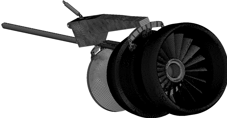
Figure 2: FEA model: Generic fan rig model
