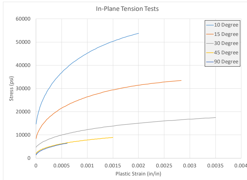
Fig. 3.10. 1-2 plane tension stress-plastic strain curves at off-axis angles of \theta = 10^\circ, 15^\circ, 30^\circ, 45^\circ , and 90^\circ
