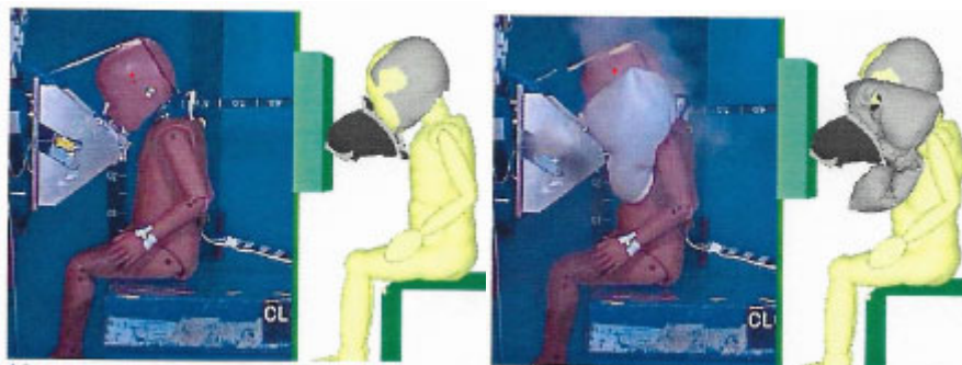
Figure 6-34 Folded Airbag Comparison
