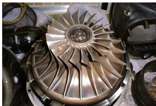
Figure 5-9 APU Compressor Rotor
