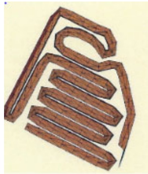
Figure 6-41 Folded Airbag CAD
